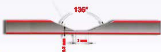
V-Shaped Groove for 45° folding
